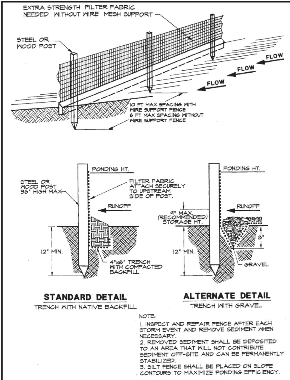
**Figure 4.4a. Silt Fence**
