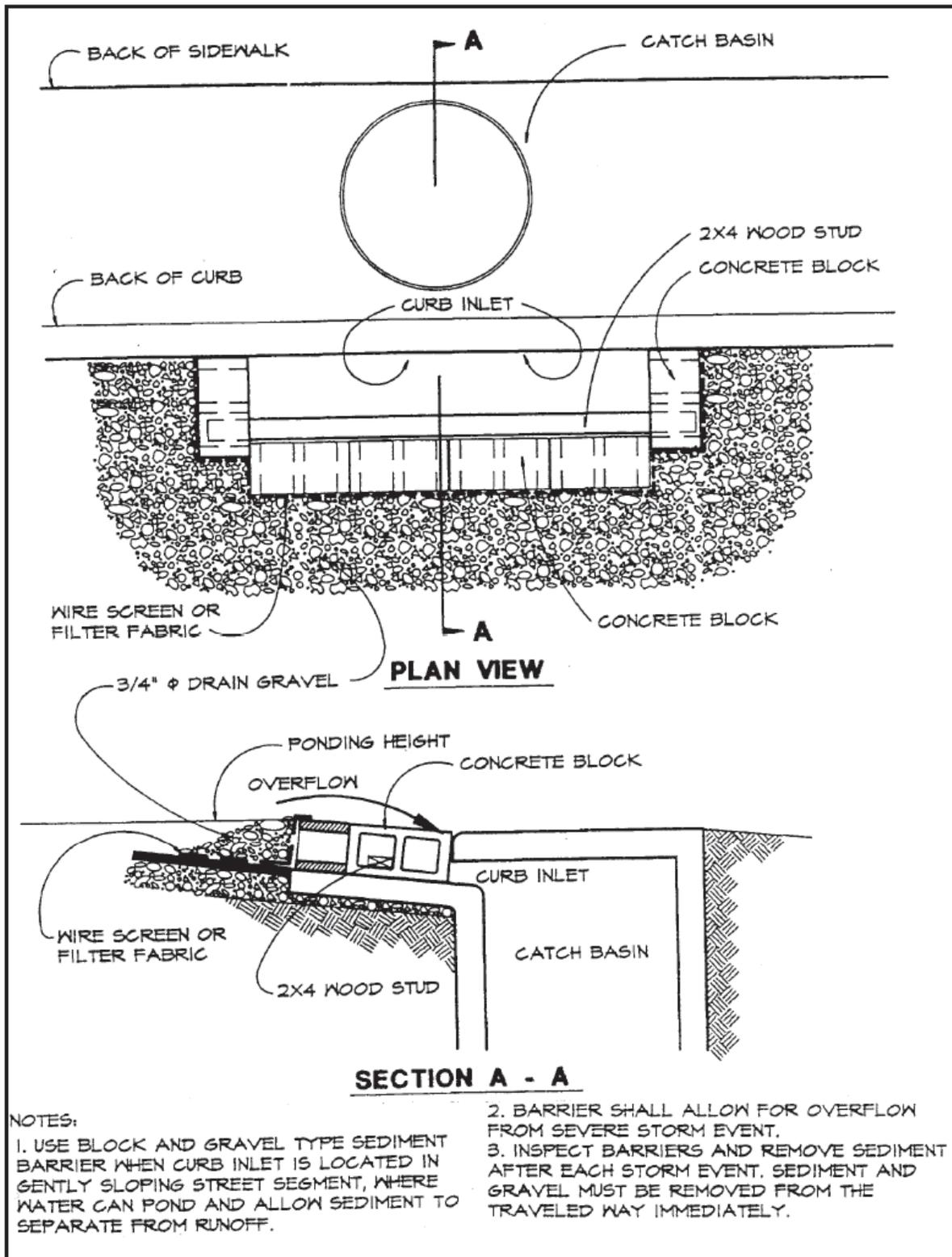
**Figure 4.5i. Block and Gravel Curb Inlet Sediment Barrier**
