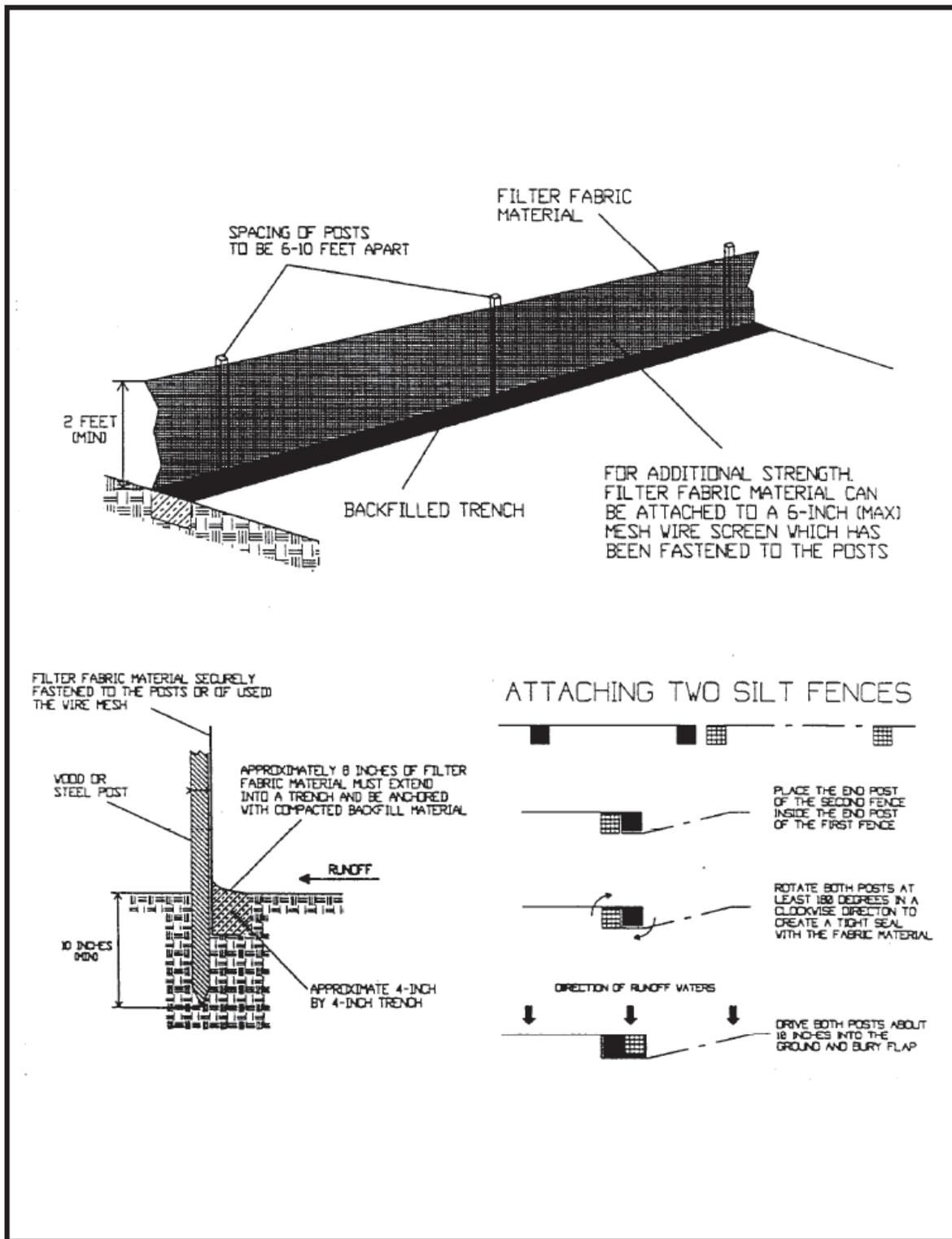
**Figure 4.4b. Installing a Filter Fabric Silt Fence**
